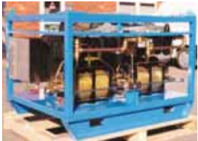
15,000 psi Glycol Injection Skid
